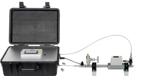
S600 with the isokinetic sampler attached
