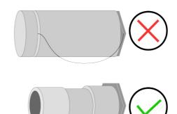
Remove the protection caps from all parts of both sides of the instrument. If not removed, the device may get damaged and the risk of bursting parts under high pressure can even lead to personal injuries. All exhaust outlets will pass air during the measurement, if not, please contact the manufacturer.
