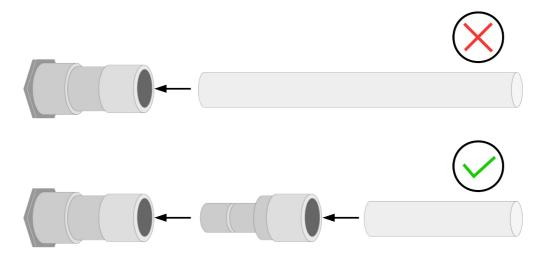
Directly plugging and pulling the teflon hose more than once may lead to particle contamination, which can affect the measurement. To avoid this problem, please use the included adapter plugs and keep them on your tubes.
